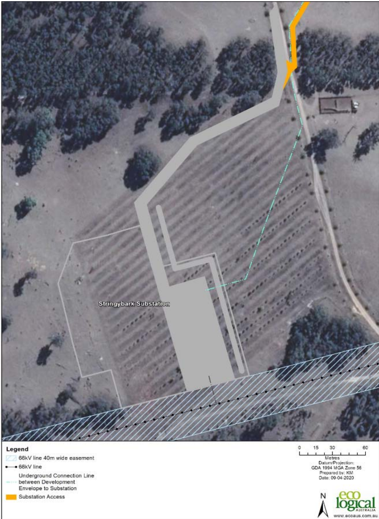
Figure 14 – Revised Olive Grove Plan indicating new underground connection cable to approved Stringybark Substation
